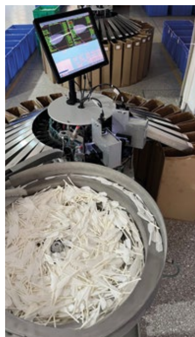
New Technologies and a high volume of raw feathers, allow RSL to sort feathers into up to 50.000 types of feathers, to find the exact matches for the perfect shuttlecock.
